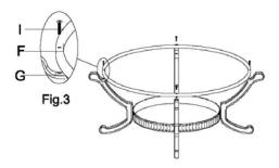
Step 4: Place the fire bowl (E), log grate (D), mesh cover (B) on the assembled base. When the appliance has cooled down COMPLETELY and NOT in use, put cove (N) on the appliance.
