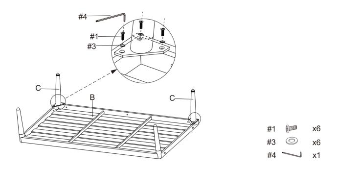
Step 2. Lay back panel (part A) down on a soft flat surface, such as carpet, as shown below.
