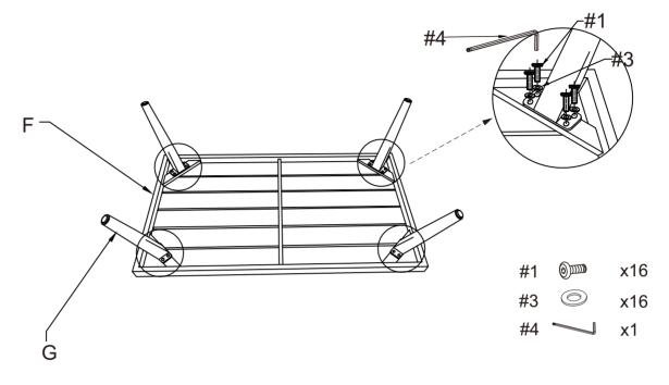
Step 5. Carefully turn assembled unit upright on a flat surface.
