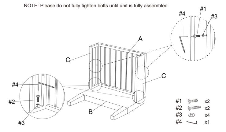
Step 3. Attach side panel (part B) to top panel (part A) and end panels (part C) using short bolts (part #1), long bolts (part #2), flat washers (part #3) and allen wrench (part #4).
