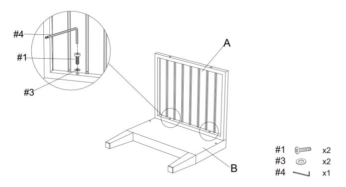
Step 2. Attach end panels (part C) to top panel (part A) and side panel (part B) using short bolts (part #1), long bolts (part #2), flat washers (part #3) and allen wrench (part #4).
