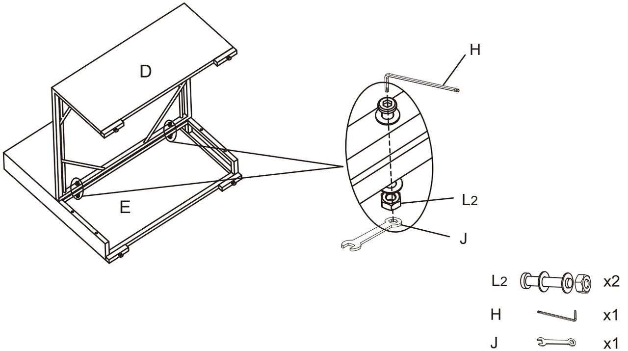
Step 5. Attach side panels (part F) to back panel (part E) and seat panel (part D) using short bolts with washers (part L1), long bolts with washers and nuts (part L2), allen wrench (part H) and wrench (part J).
