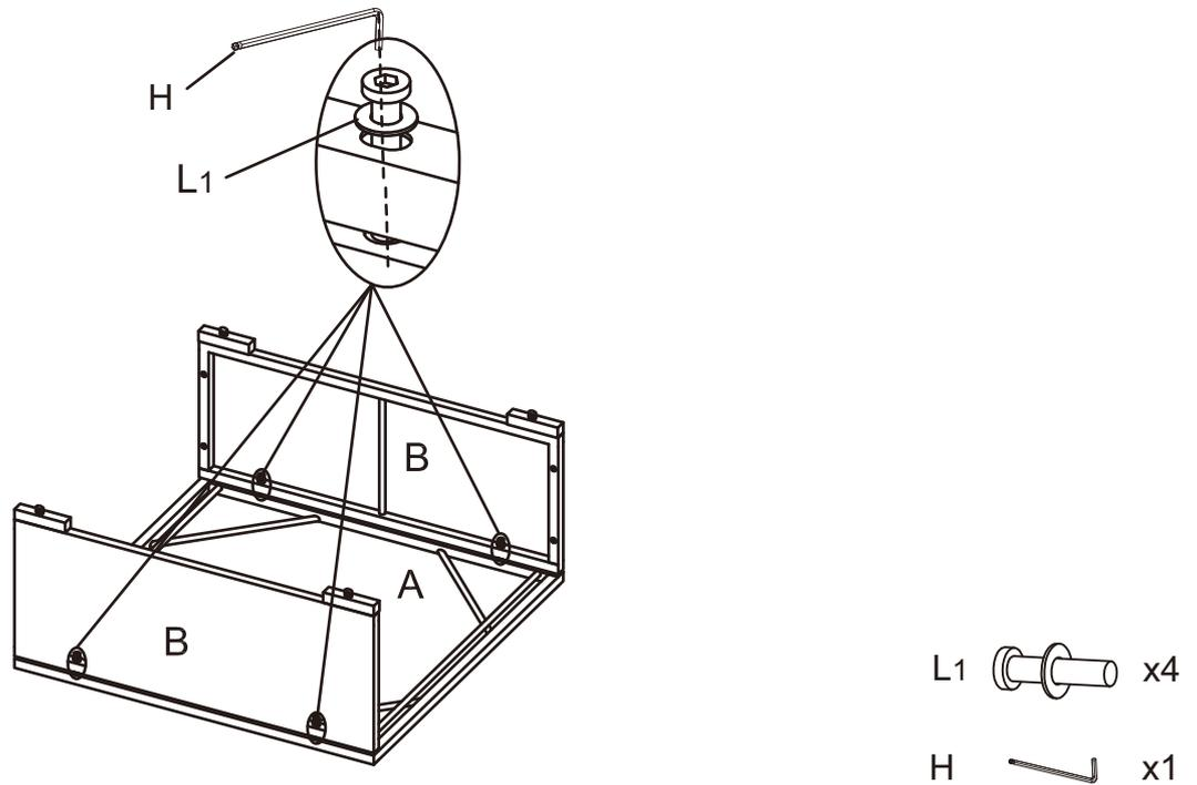
Step 2. Attach side panels (part F) to side panels (part B) using short bolts with washers (part L1) and allen wrench (part H).
