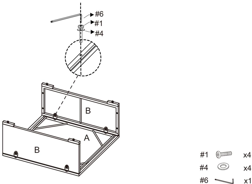
Step 2. Attach side panels (part E) to side panels (part B) and wicker top (part A) using short bolts (part #1), flat washers (part #4) and allen wrench (part #6).
