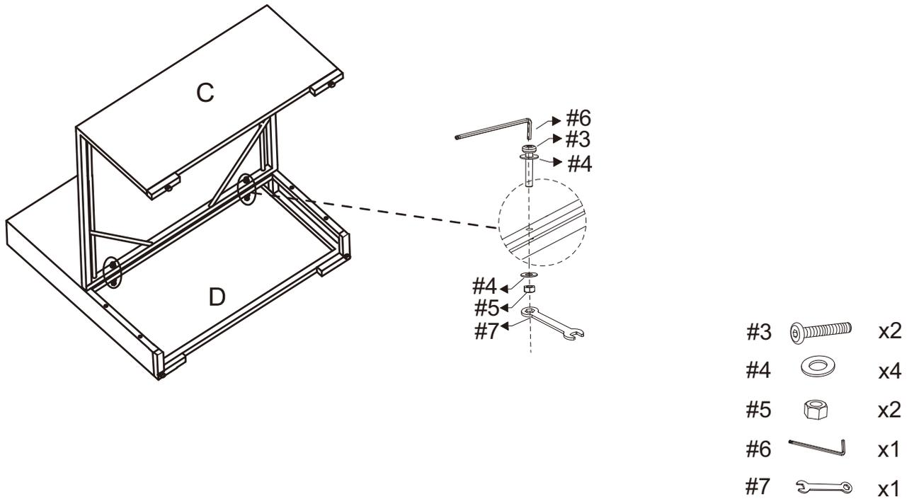
Step 5. Attach side panels (part E) to back panel (part D) and seat panel (part C) using short bolts (part #1), medium bolts (part #2), flat washers (part #4), hex nuts (part #5), allen wrench (part #6) and wrench (part #7).
