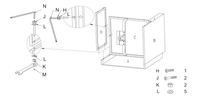
Step 4. Attach the other Arm panel(A) to the assembled Parts (A,B,C&D) using Medium Bolts (I),Long Bolts (J),Washers (L),Nuts (K),Wrench (M) and Allen Key (N) as shown.
