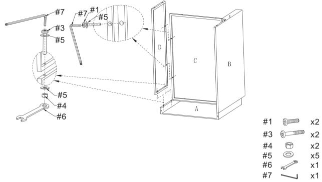
Step 4.Attach arm panel (part A) to assembled unit (parts A,B,C&D) using medium bolts (part #2),long bolts (part #3), washers (part #5),nuts (part #4),wrench (part #6)and allen key (part #7).
