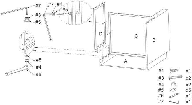
Step 4. Attach arm panel (part A) to assembled unit (parts A,B,C&D) using Medium bolts (part #2), long bolts (part #3), washers (part #5), nuts (part #4), wrench (part #6) and allen key (part #7).
