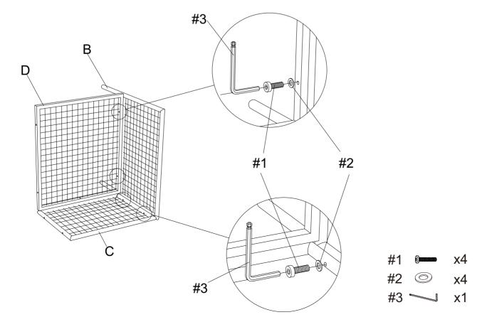
Step 3. Attach right arm panel (part A) to seat panel (part D) and back panel (part C) using bolts (part #1), flat washers (part #2) and allen wrench (part #3).
