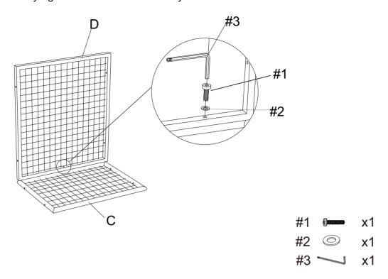
Step 2. Attach left arm panel (part B) to back panel (part C) and seat panel (part D) using bolts (part #1), flat washers (part #2) and allen wrench (part #3).
