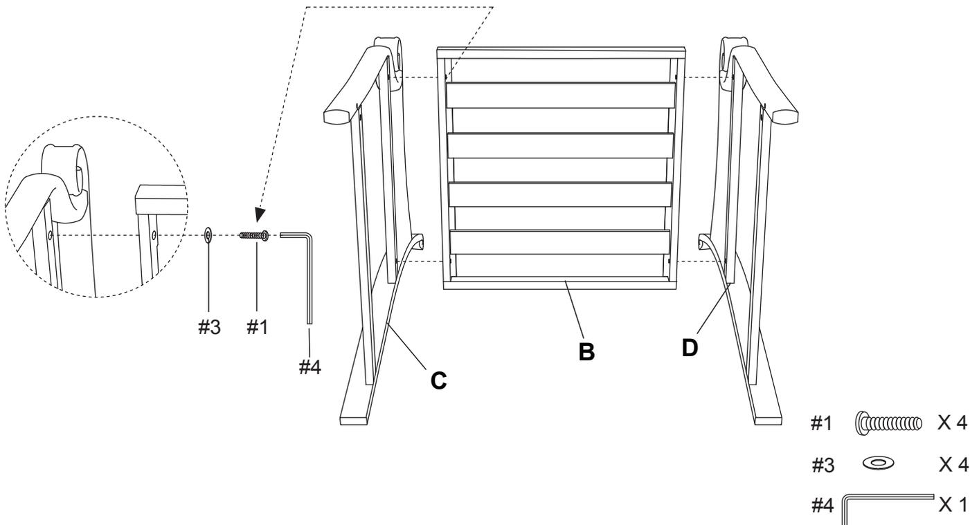
Step 2. Attach back panel (part #A) to arms (part #C&D) using long bolts (part #1), washers (part #3) and allen key (part #4)
