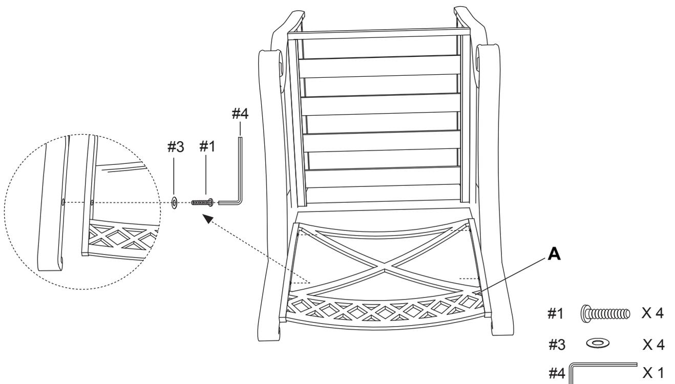
Step 3. Attach foot support (par #E) to front leg using short bolts (par #2), washers (part #3) and allen key (part #4)
