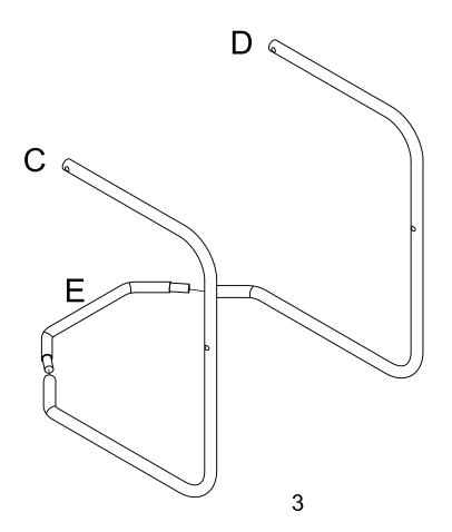
Step 3. Attach support legs (parts C & D) to chair back (part A) and chair seat (part B) using long bolts (part #1), Round Plastic Washer (part #8), hex nuts (part #3), flat washers (part #4), plastic washers (part #7), wrench (part #5) and allen wrench (part #6).
