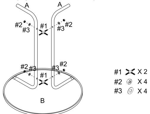
Step 2. Attach remaining support legs (part A) to assembled unit (parts A & B) using nuts (part #2), washers (part #3) and wrench (part #5). Add tube caps (part #4) to support legs (part A).
