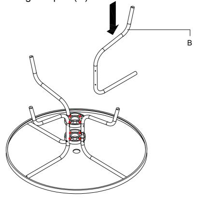
STEP 7 Attach the fourth Leg (B) to the Leg Coupler (C) using Allen Bolts (Part#1) and Flat Washers (Part#2) as shown.
