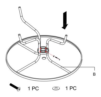
STEP 5 Attach the second Leg Coupler (C) to the three Legs (B) using Allen Bolts (Part#1) & Flat Washers (Part#2) as shown.
