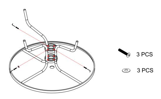
STEP 6 Add the fourth Leg (B) by fitting the flat end of the leg under the lip of the table and positioning the portion with the bolt holes into the Leg Coupler (C).
