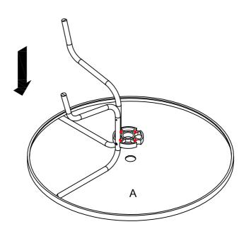
STEP 4 Add a third Leg (B) fitting the flat end under the lip of Top (A) and attach using an Allen Bolt (Part#1) and Flat Washer (Part#2) as shown.
