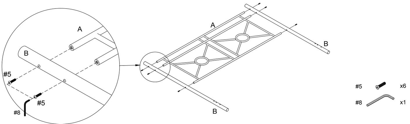
Step 2. Lay panel (part A) upside down on a soft flat surface, such as carpet, as shown below. Attach footboard legs (part C) to panel (part A) using long sunk bolts (part #5) and allen wrench (part #8).
