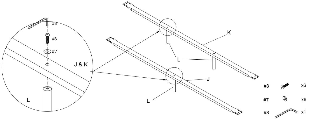
Step 5. Attach assembled units (parts J, K & L) to side rails (part I) using bolts (part #1), flat washers (part #7), hex nuts (part #6), allen wrench (part #8) and wrench (part #9).
