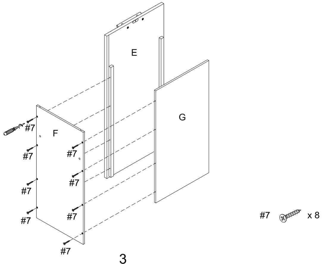
Step 3. Attach box side panel (part F) to assembled unit (parts E & G) using long screws (part #7) and phillips head screwdriver.
