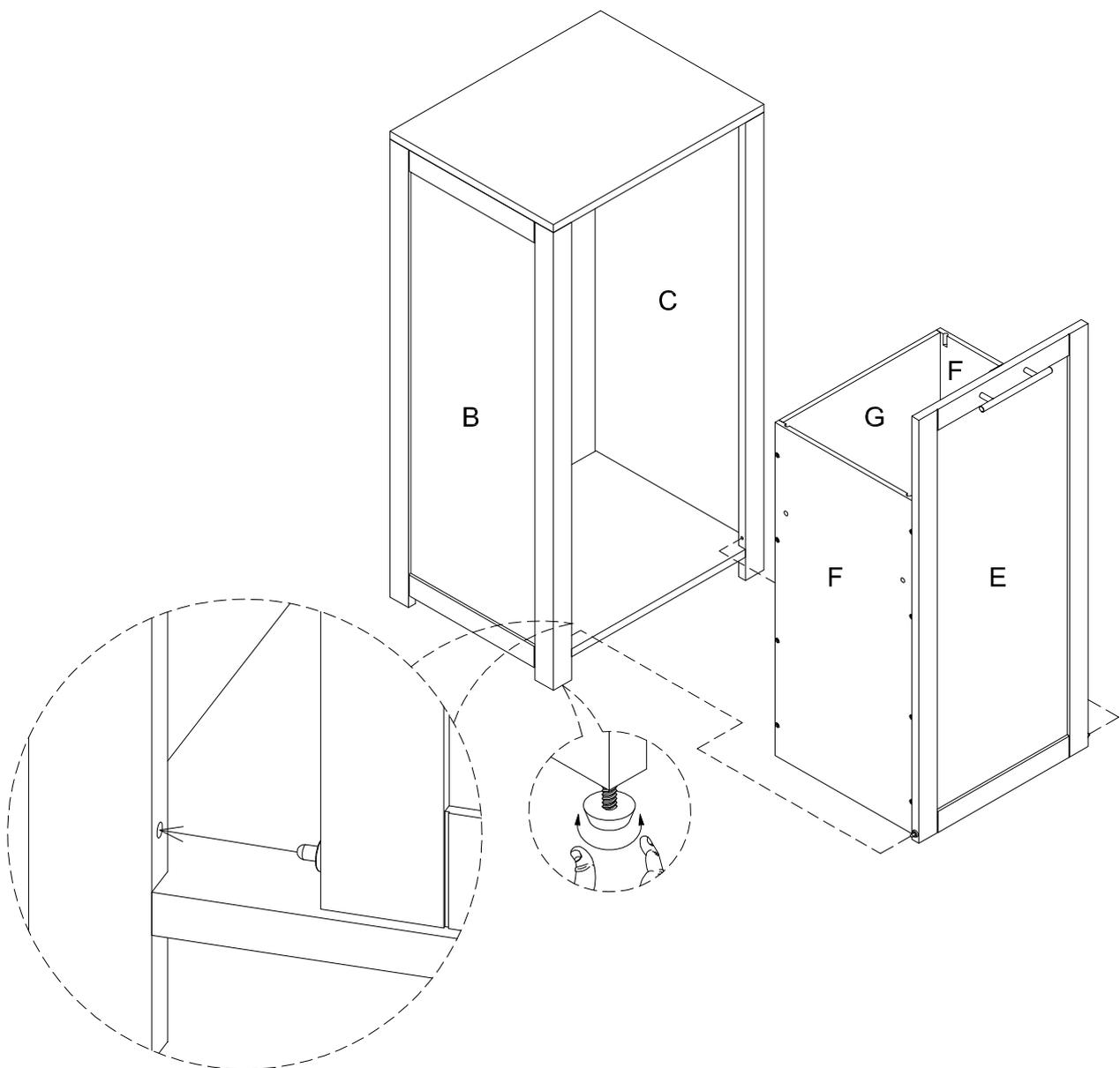
Step 9. Insert wood dowels (part #2) into box side panels (part F).
