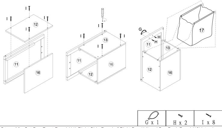
Step 10. Set Box Front Panel (11), Right Side Panel of Right Box (14) and Box Back Panel (16) into place using Long Screw (I). Attach Left Side Panel of Right Box (15) into place using Long Screw (I). Attach Handle (G) to Box Front Panel (11) using Round Head Bolt (H). Place Bag (17) into box and secure by inserting rods into predrilled holes.
