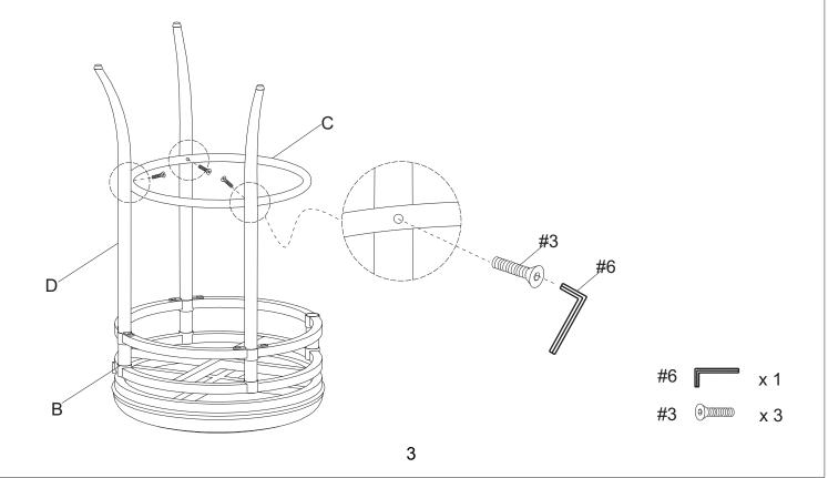
Step 3: Attach remaining leg (part D) to seat (part B) and footrest ring (part C) using short bolts (part #1), long bolt (part #3), spring washers (part #4), flat washers (part #5) and allen wrench(part #6).
