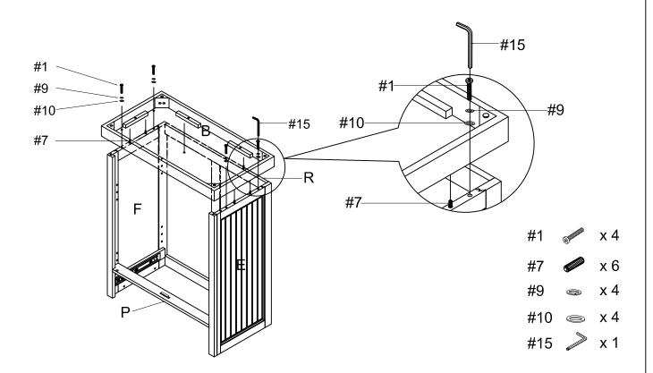
Step 7. Attach the assembled top and bottom cabinets using short hex socket head bolts (part #2), spring washers (part #9), flat washers (part #10) and allen wrench (part #15).
