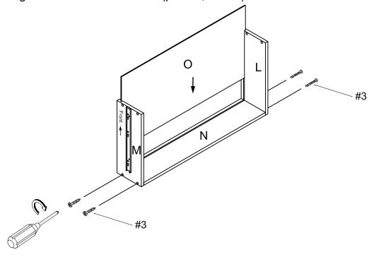
Step 12. Attach drawer front panel (part K) to assembled unit (parts L, M & O) using long flat head screws (part #3) and phillips head screwdriver. Attach handles (part #12) to drawer front panel (part K) using handle bolts (part #5) and phillips head screwdriver.
