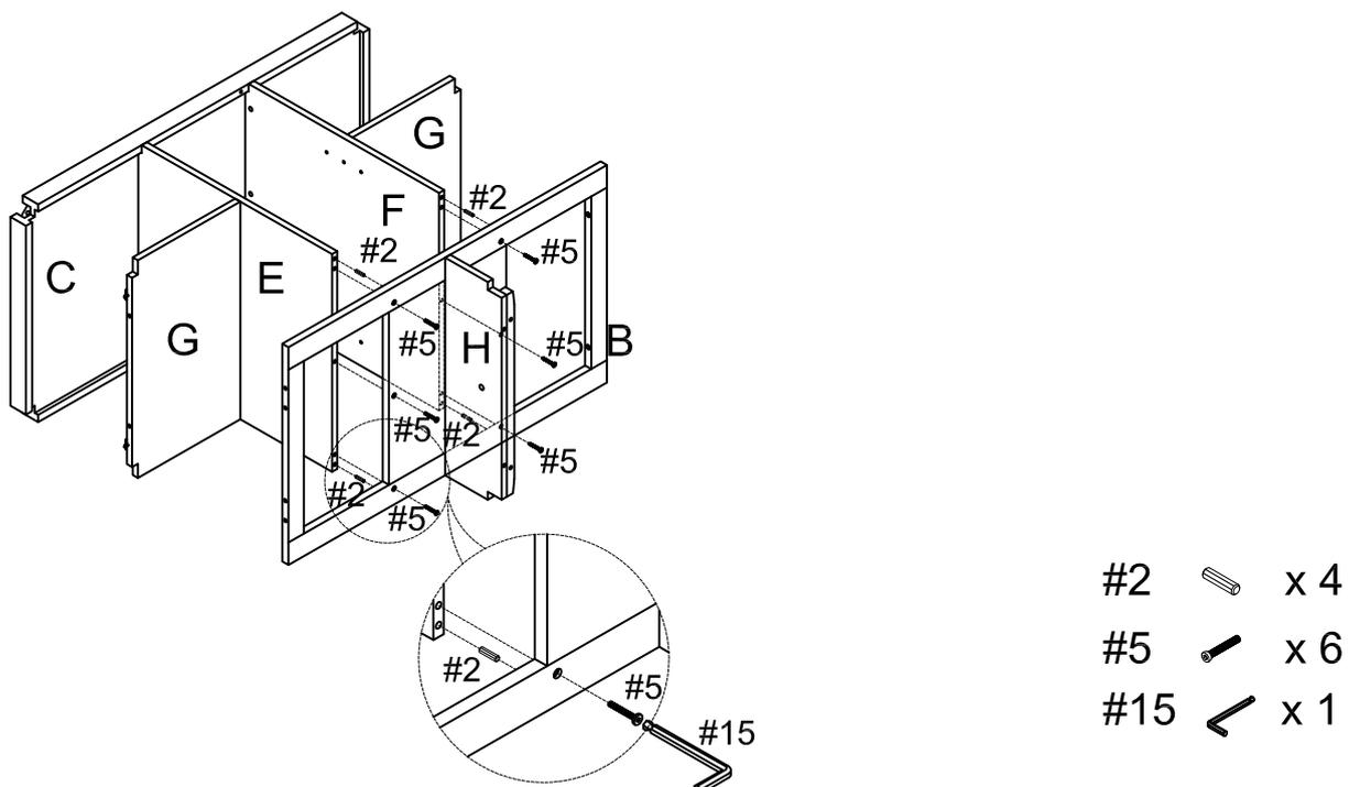
Step 6. Place top rails (part K) on drawer partition panel (part H). Attach side frame (part D) to assembled unit (parts B, C, G & K) using medium wood dowels (part #2), flat washers (part #8), spring washers (part #9), long bolts (part #6), allen wrench (part #15) and lock the hardware.
