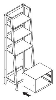
Step 11. Attach cabinet box to bookcase by using allen bolts (part #3) and allen wrench (part #4). Tighten all allen bolts at this time.
