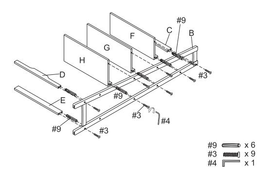
Step 9. Attach left side frame (part A) to back top rail (part C), top shelf (part F), middle shelf (part G), bottom shelf (part H), front bottom rail (part D) and back bottom rail (part E) by using large wood dowels (part #9), allen bolts (part #3) and allen wrench (part #4). Note: Do not completely tighten all allen bolts (part #3), until later on.
