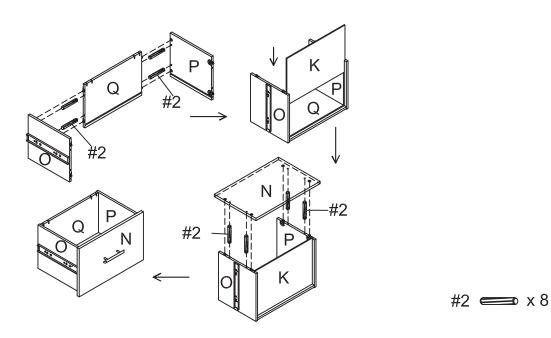
Step 3. Insert aluminum rods (part #8) into desired place in drawer.
