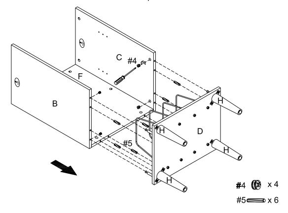
Step 6. Carefully turn unit upright. Insert cam locks (part #4) into the pre-drilled holes on the bottom of back panel (part F) and lock using phillips head screwdriver.
