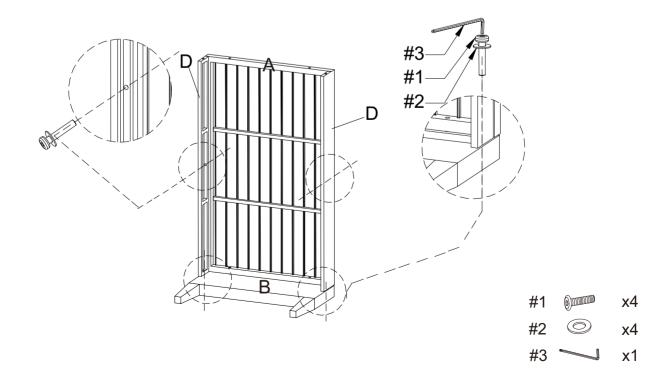
Step 3. Attach right panel (part C) to side panels (part D) and top panel (part A) using bolts (part #1),
