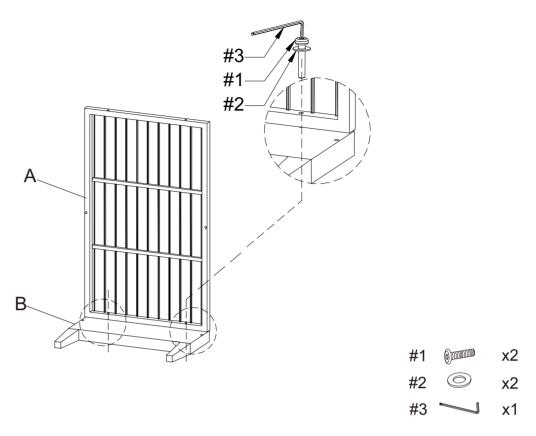
Step 2. Attach side panels (part D) to left panel (part B) and top panel (part A) using bolts (part #1), flat washers (part #2) and allen wrench (part #3).
